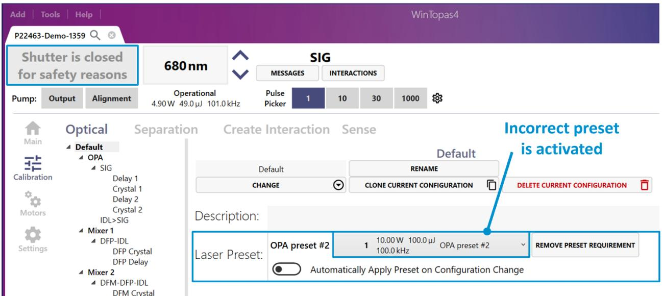
Figure 61. Closed shutter due to incorrect activated pump laser preset in WinTopas4
