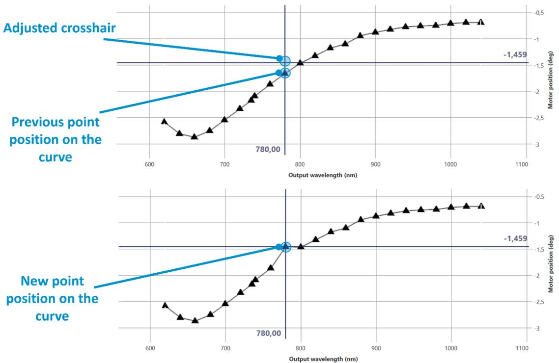
Figure 22. Adjustment of the motor position on the calibration curve in WinTopas4
