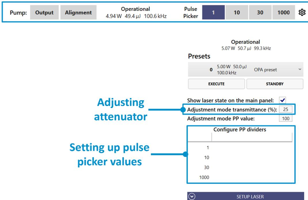
Figure 59. Adjusting attenuator and pulse picker values of the pump laser in WinTopas4
