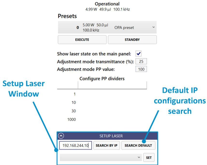
Figure 60. Pump laser setup in WinTopas4
