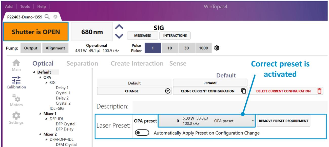
Figure 62. Opened shutter with correct pump laser preset being activated in WinTopas4
