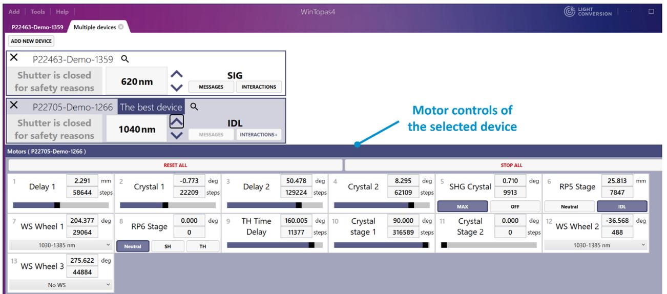
Figure 51. Multiple devices window interface with controls of the device in WinTopas4
