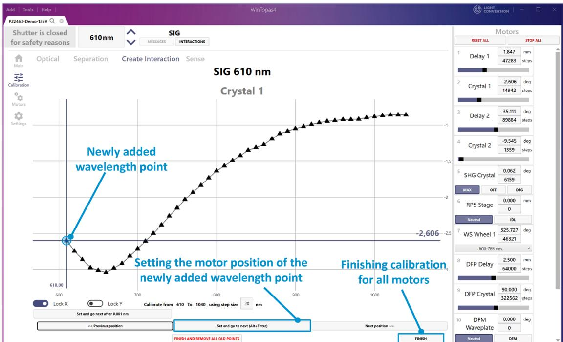
Figure 31. Motor calibration after extending interaction range in WinTopas4
