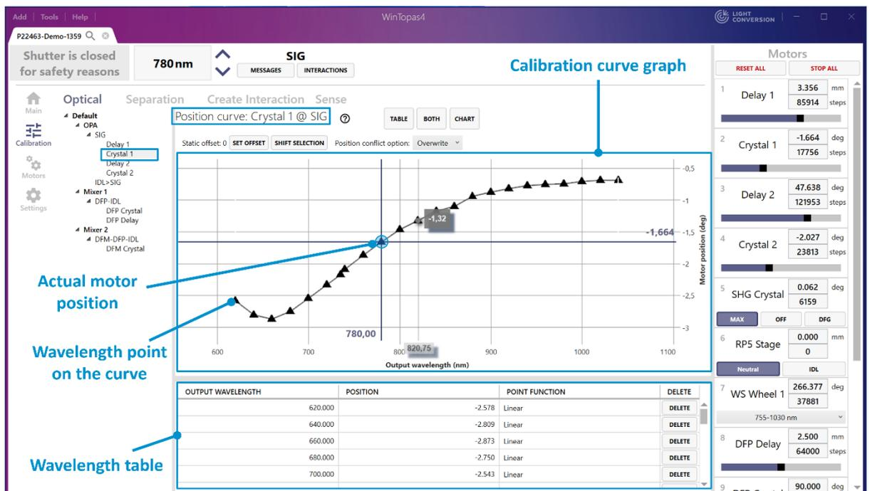
Figure 20. WinTopas4 Signal interaction motor “Crystal 1” calibration curve
