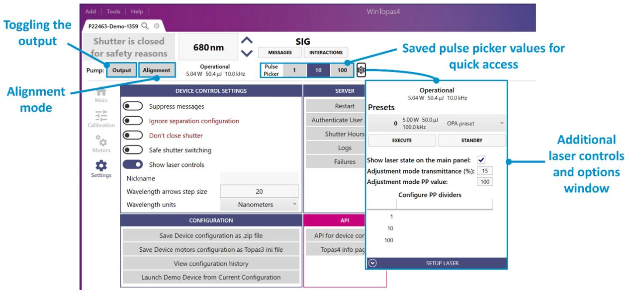
Figure 57. Controls, indicators and options of a pump laser in WinTopas4
