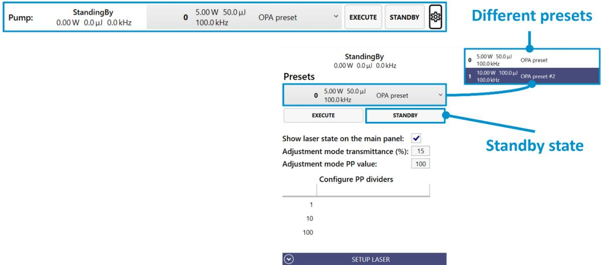
Figure 58. Standby state of the pump laser in WinTopas4
