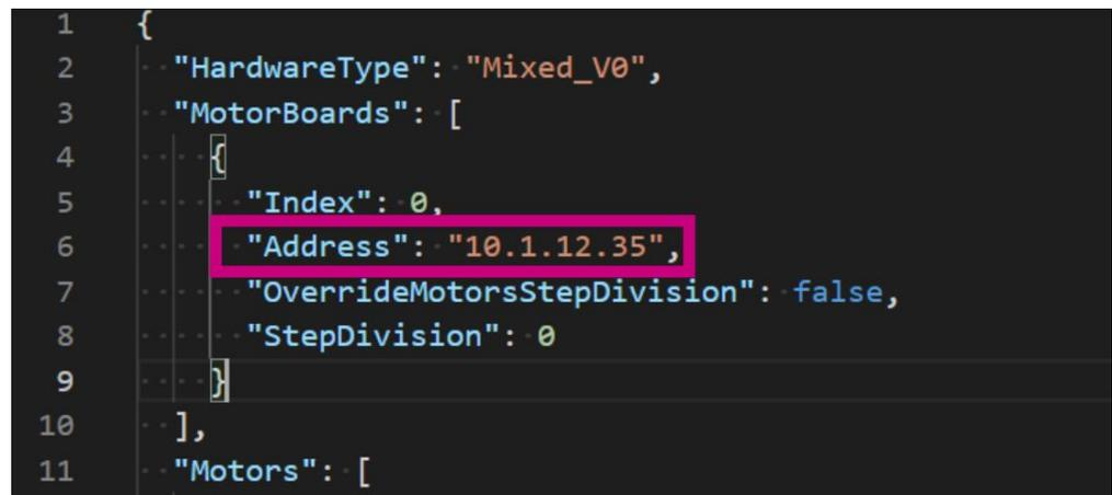
Figure 8. Motor boards configuration using text editor
